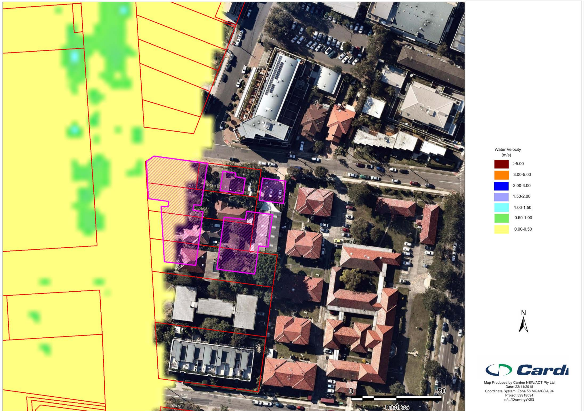
Figure 8 PMF Velocities under Existing Conditions
