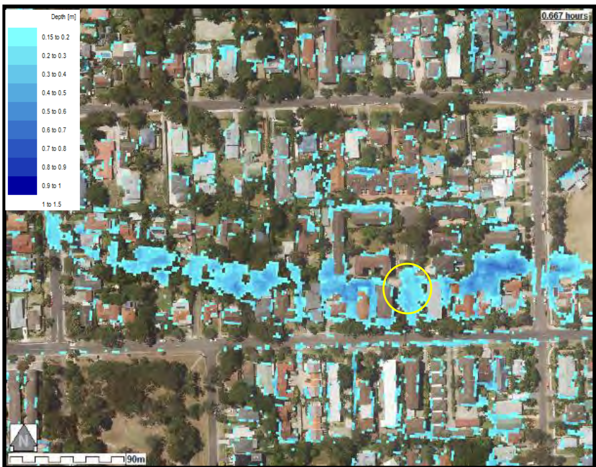
Plate 39 1% AEP Depths between King and Bishop Street after 40mins of rainfall showing significant depths forming within properties and isolating properties requiring access from Woolcott Street.
