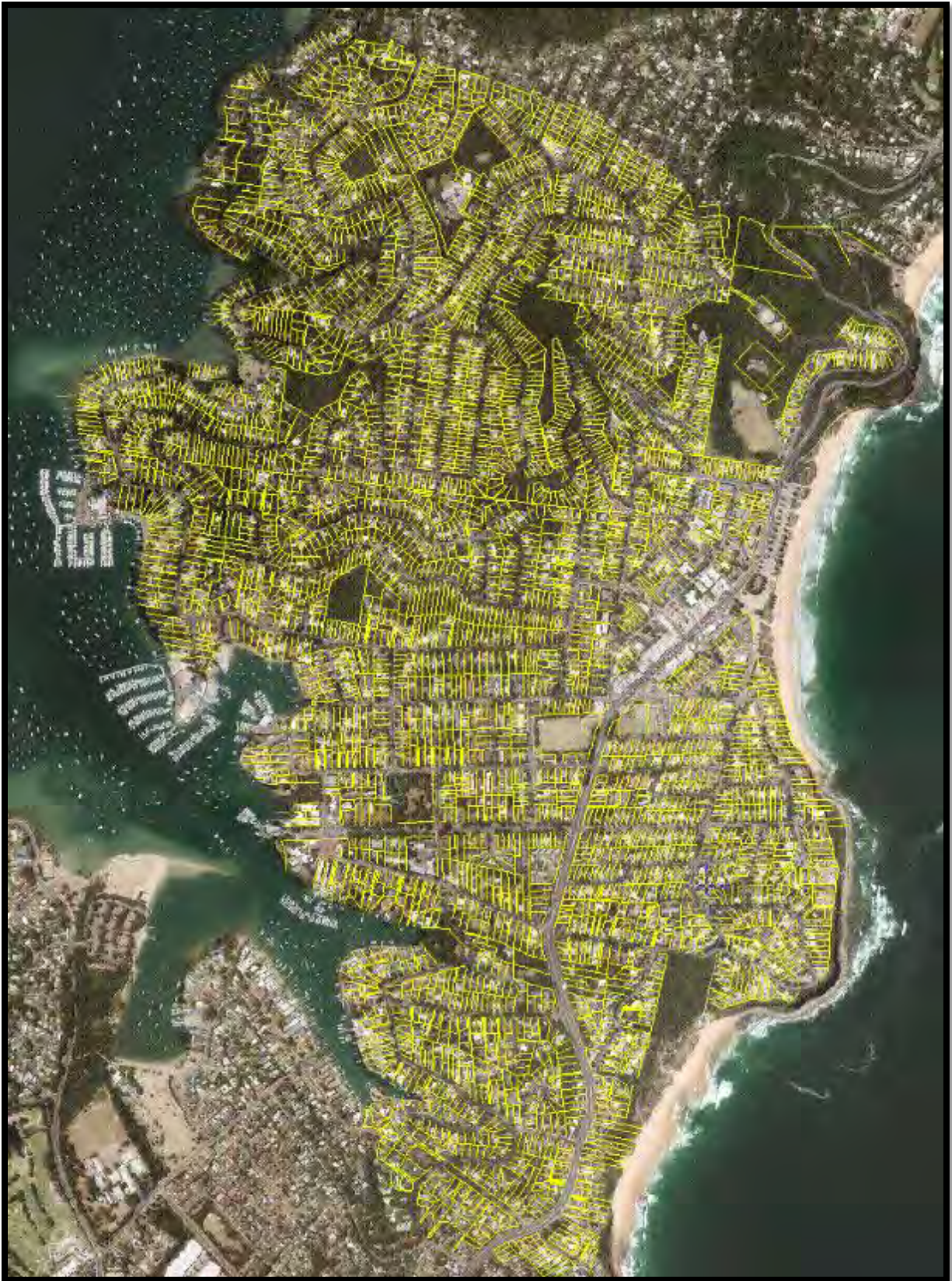
Plate 14 Extent of fences (yellow lines) extracted using cadastre, zoning and roadway GIS layers
