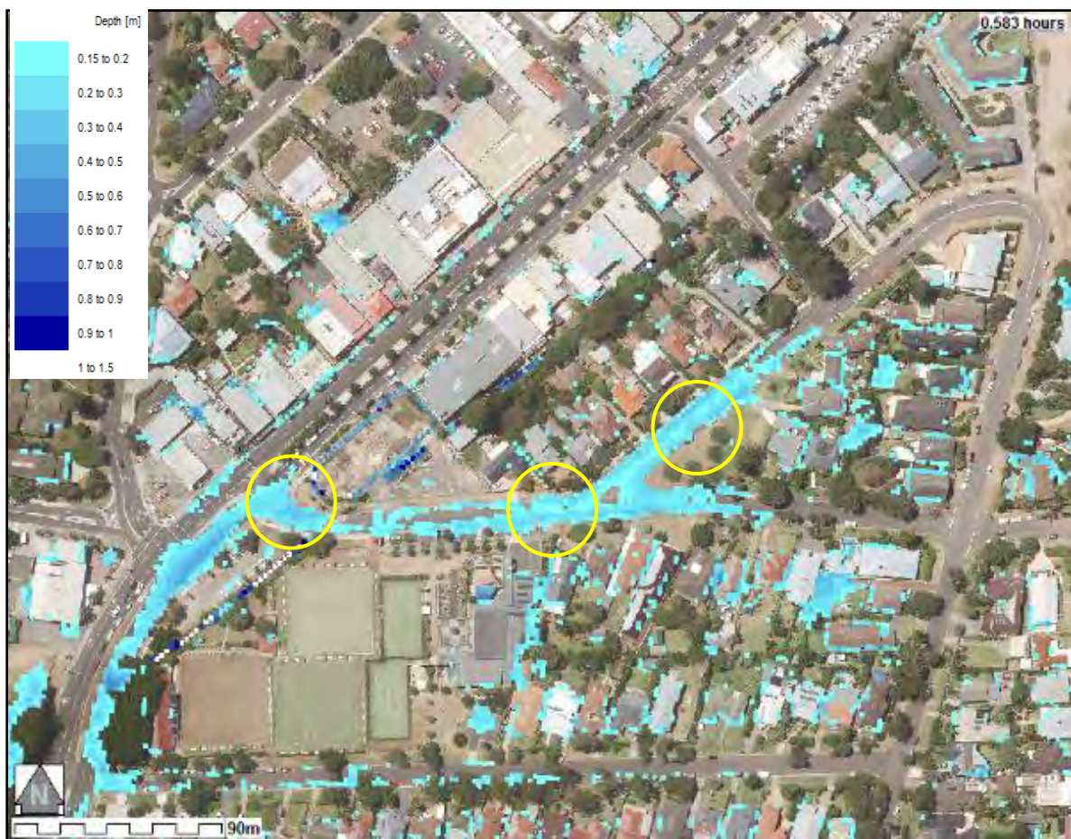
Plate 37 1% AEP Depths in vicinity of Ross Street and Bramley Avenue after 35mins of rainfall showing multiple roadway cut locations.
