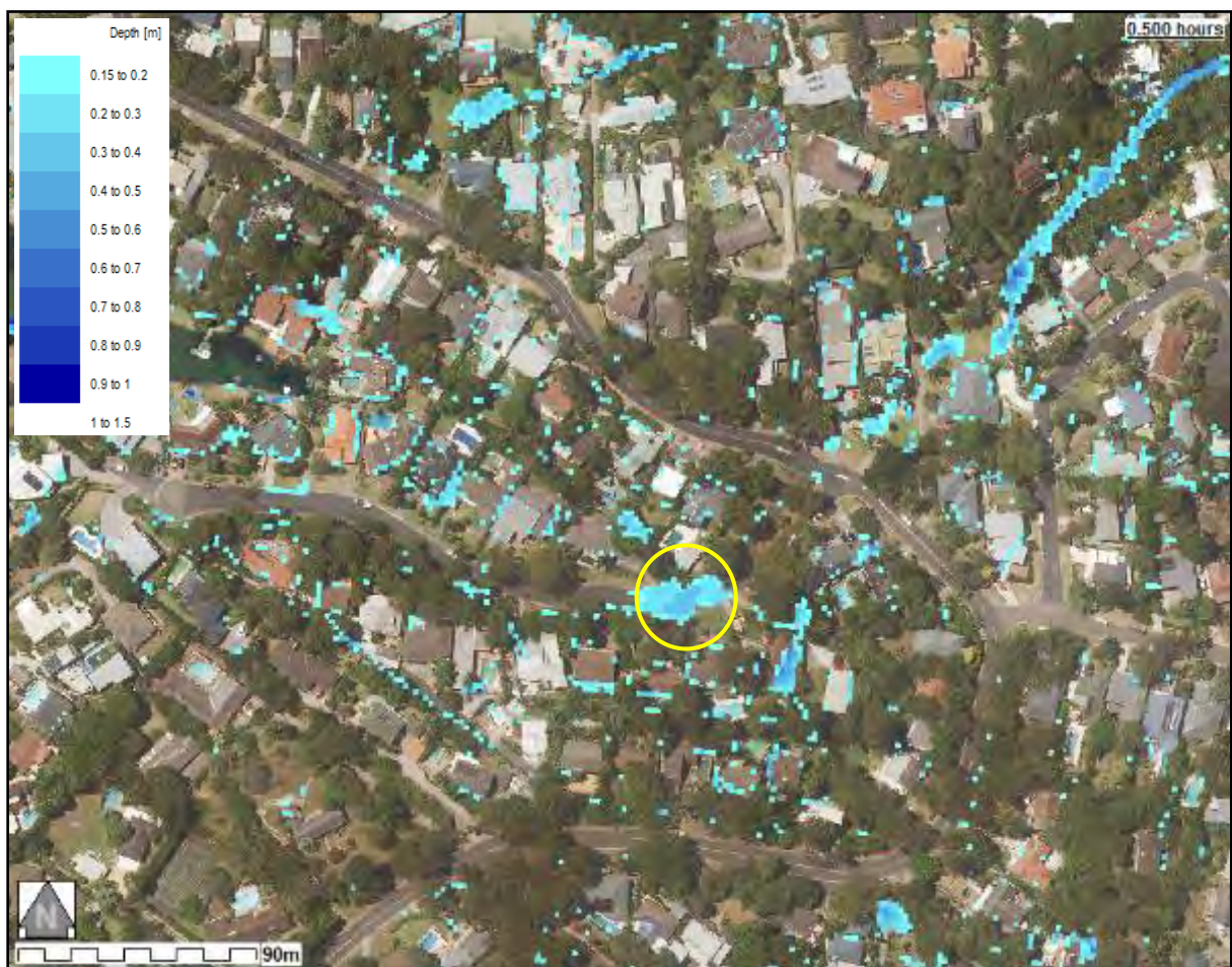
Plate 38 1% AEP Depths in vicinity of Yachtsmans Paradise after 30mins of rainfall showing significant depths forming on the roadway and isolating properties requiring roadway access.
