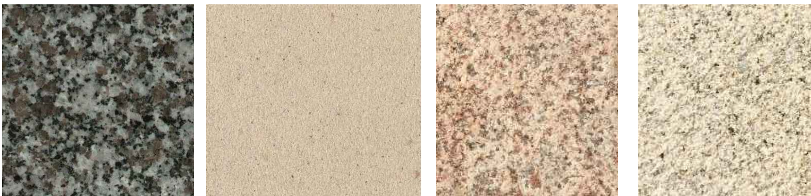
Proposed Granite Plinth, Granite Setts, Granite Edge (Harcourt Grey) Proposed Columbarium Wall (Sandy Yellow Granite - Exfoliated Finish) Proposed Columns (White Sandstone) Proposed Granite Rock Faced Capping (Sandy Yellow Granite - Bush Hammered)
