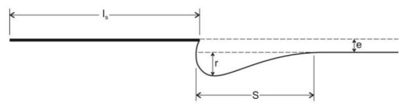
Figure 14: Seawall end effect variables
