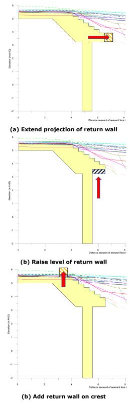
Figure 13: Options for reducing wave overtopping
