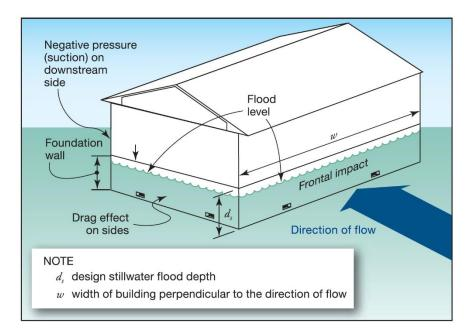
Figure 11: Hydrodynamic loads on a building [Source: FEMA, 2011]
