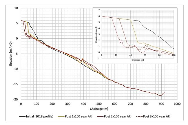
Figure 3: Evolution of beach profiles for consecutive storms in SBEACH with no seawall in place
