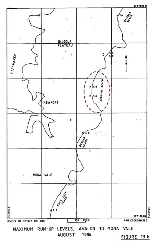
Figure 6: Observed wave runup levels after August 1986 storm based on debris lines [Source: Higgs and Nittim, 1988]
