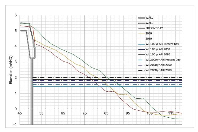
Figure 5: Water levels (no wave setup) for 100 and 2000 year ARI events for present day, 2050 and 2080 planning period
