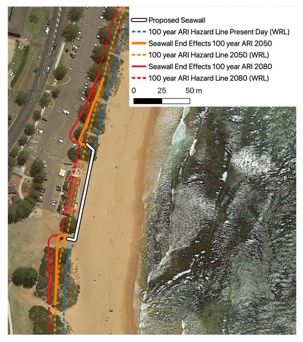
Figure 15: Theoretical seawall end effect for 100 year ARI conditions
