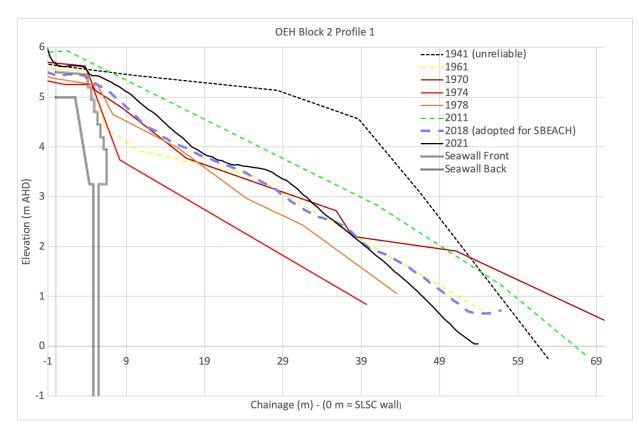
Figure 1: Measured profile data with proposed seawall superimposed
