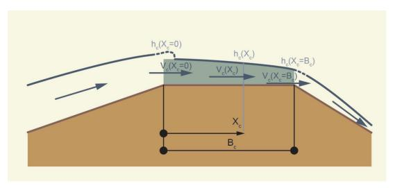
Figure 10: Sketch of overtopping flow parameters [Source: EurOtop, 2008]
