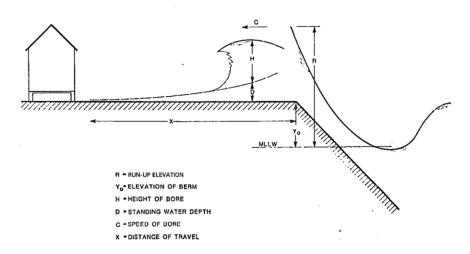
Figure 9: Definition of overtopping parameters [Source: Cox and Machemehl, 1986]
