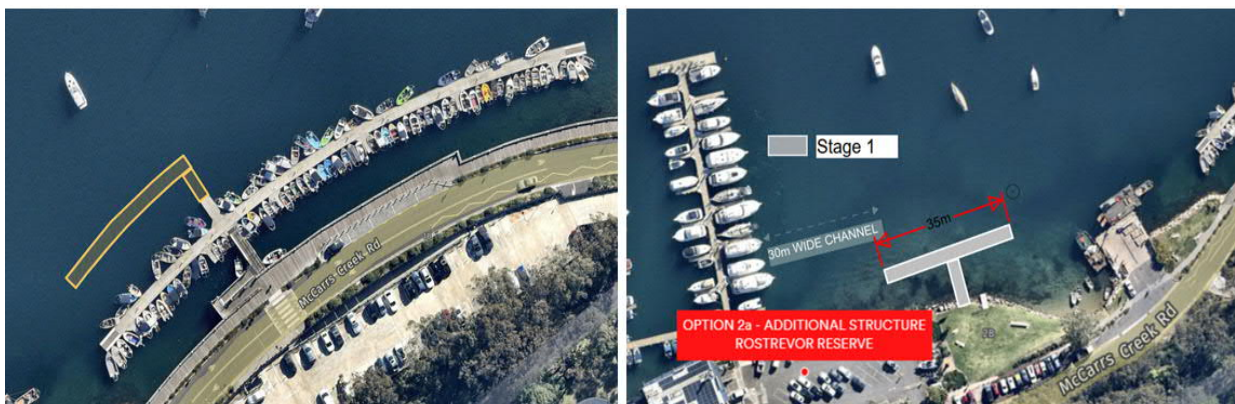
Figure 3-11 Option 4 Combining Stage 1 of Option 1b and 2a. Providing an Additional 66 Berths and 177 in Total.
