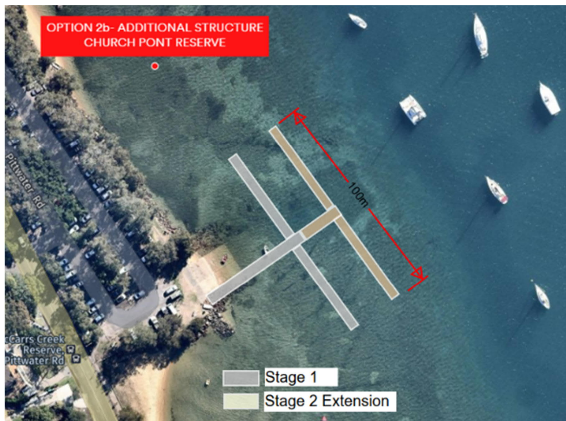
Figure 5-7 Option 2b Staged Concept Floating Pontoons Church Point Reserve.
