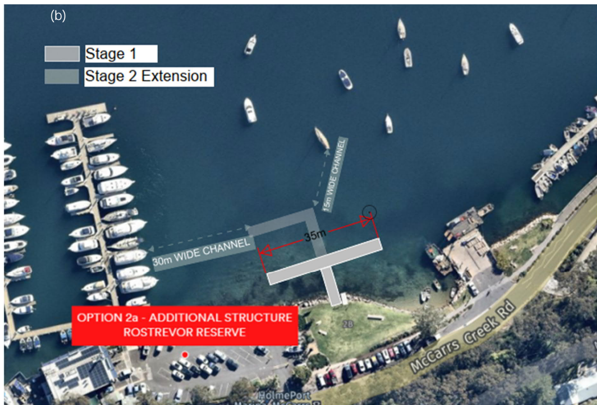
Figure 3-4 Option 2a Staged Concept Floating Pontoons Rostrevor Reserve. (a) Initial Concept Option 2a Presented to Stakeholders and (b) Revised Concept Options 2a With Stage 1 Additional 32 Boat Berths and Stage 2 Additional 25 Boat Berths After Relocation of Swing Moorings.
