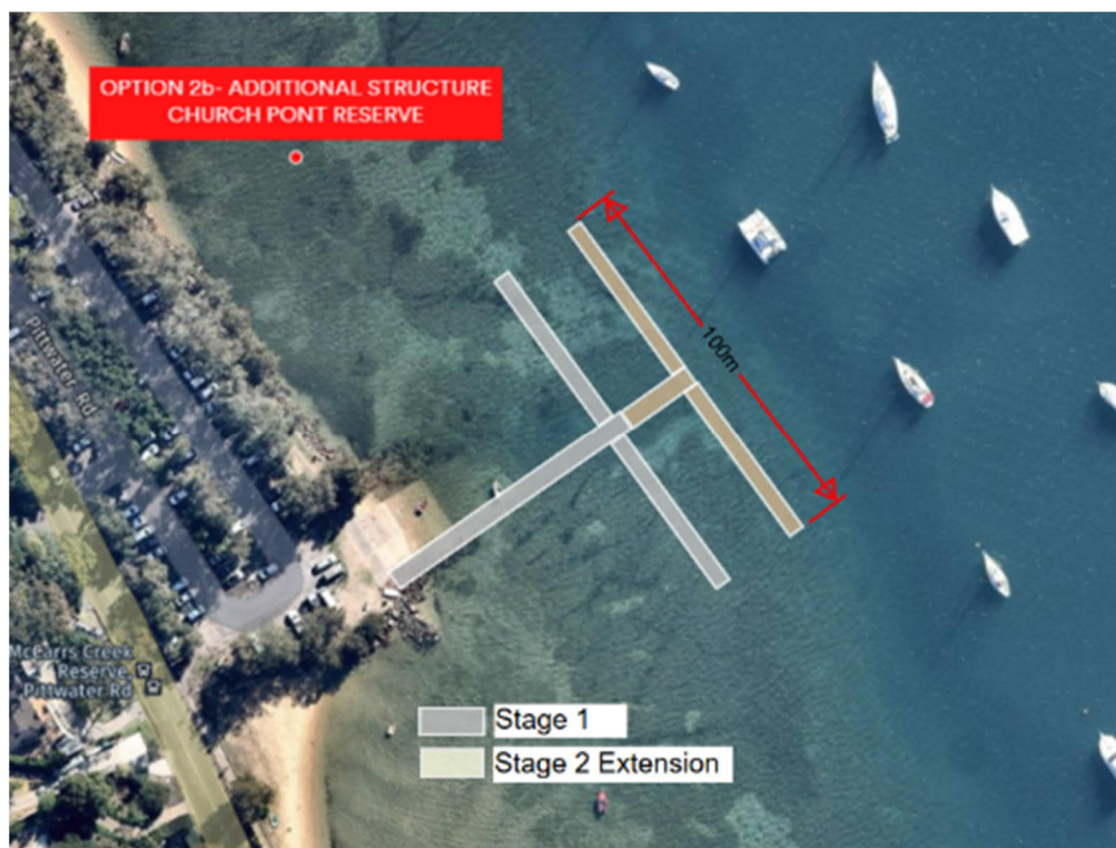
Figure 3-5 Option 2b Staged Concept Floating Pontoons Church Point Reserve. Stage 1 Additional 90 Boat Bays and Stage 2 Additional 90 Bays.
