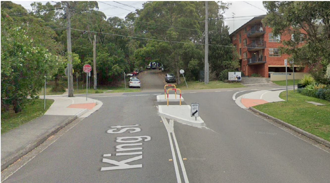
Safer Crossing Treatment Example Bent out crossing with refuge (King Street, Newport)
