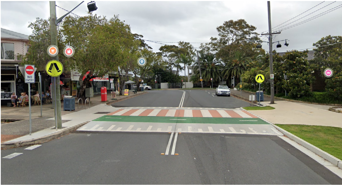
Safer Crossing Treatment Example Raised Pedestrian and Cycleway Priority Crossing (Kalinya Street, Newport)
