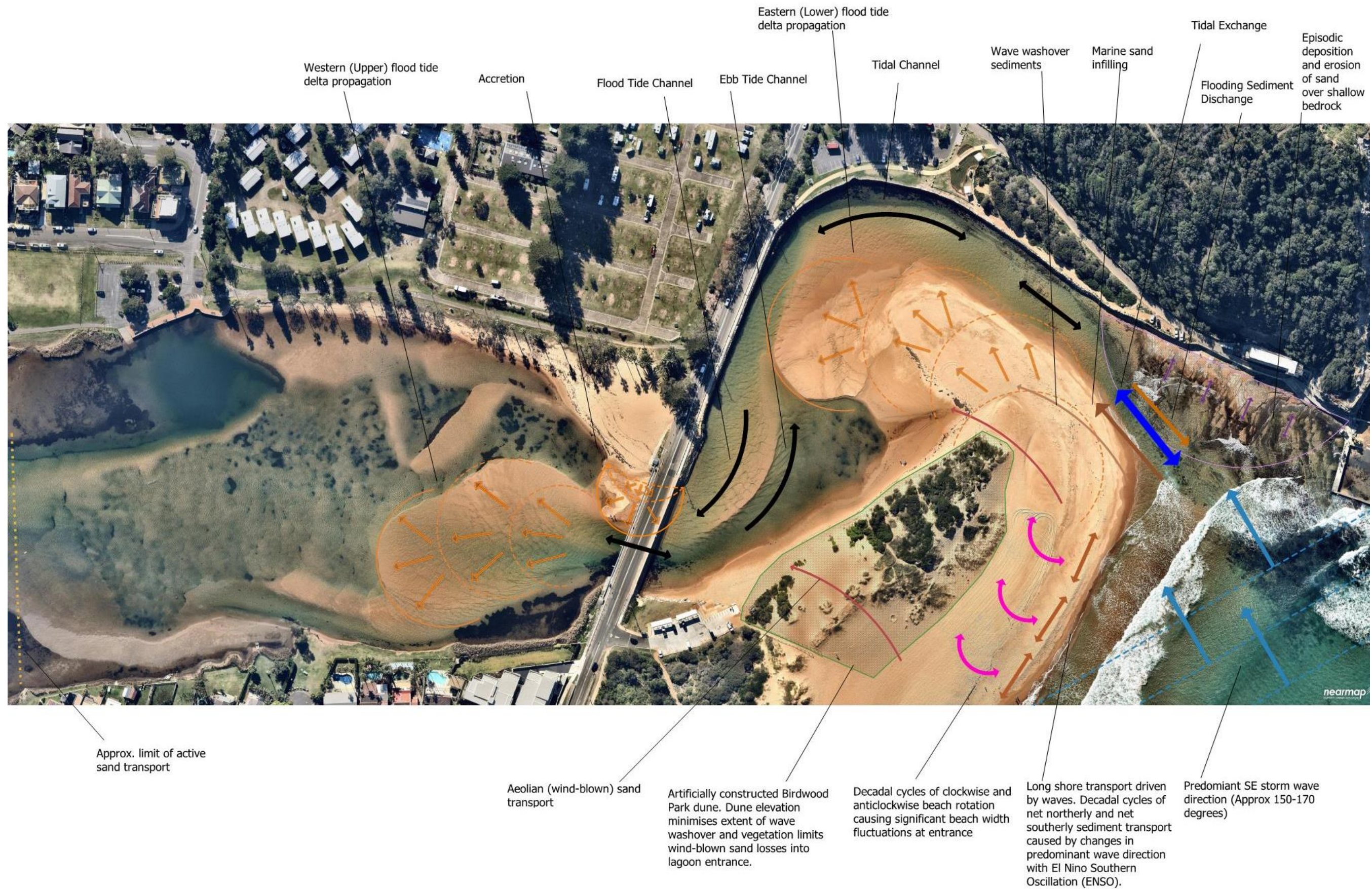
Figure 2-6: Conceptual understanding of coastal processes at Narrabeen Lagoon entrance
