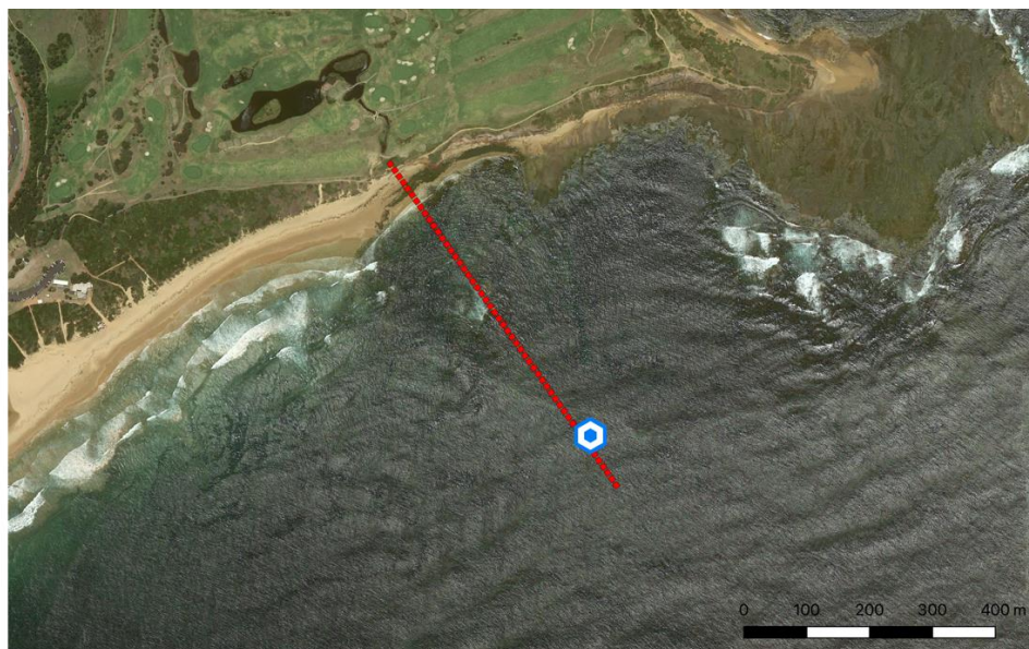
Figure 4-2 Location of the nearshore wave transformation output (blue hexagon) relative to WRL 2D idealised profile used for wave runup calculations (Aerial photo 03/12/2018; Source: Google Earth)
